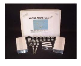
Each Marine Algaltoxkit contains all the materials to perform two 72h growth inhibition tests
