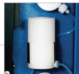
Reagent mixing chamber allows automated online reagent blending in the method
