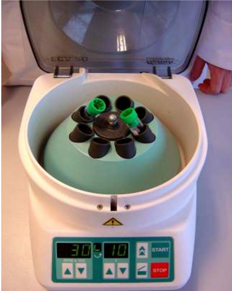
CENTRIFUGE THE TUBE FOR 10 MINUTES
