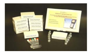
Each kit contains all the materials and reagents required to perform low-cost toxicity analysis of 10 - 20 water samples
